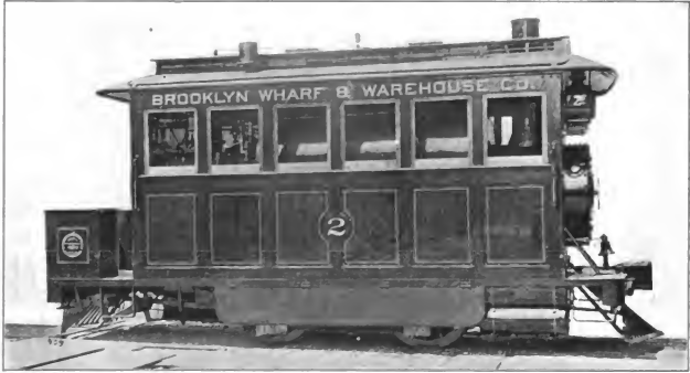
Fig. 7. Four-Wheel (0-4-0) Compound Switching Locomotive. Built by the Baldwin Locomotive Works for the Brooklyn Wharf & Warehouse Co. Cylinders 10 in. and 17 in. x 24 in., Working Steam Pressure 180 lbs. per sq. in., Heating Surface 676.56 sq. ft., Diameter of Drivers 44 in., Weight on Drivers 78,770 lbs., Total Weight 78,770 lbs.
